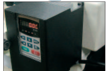
Detail of frequency converter
