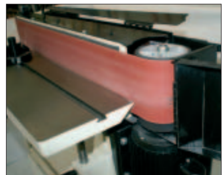
Main table tilts with the sanding head for use as a fence in the horizontal position
